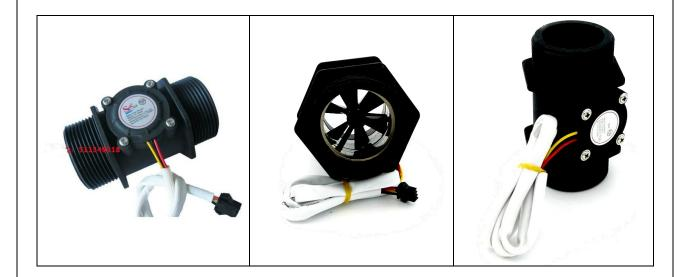
Water flow sensor is mainly composed of plastic valve body, flow of rotor components and hall sensor. It is installed in the water heater inlet, used to detect water flow, when the water through flow rotor components, Magnetic rotor rotation and speed changes with the flow, hall sensor output pulse accordingly Signal feedback to the controller by the controller to judge the size of the water flow, adjust and control.
